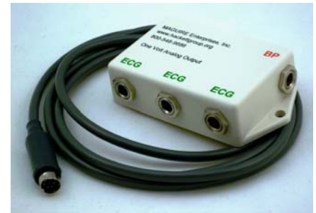
An output adapter that provides four 1/4" phone jacks (three ECG and one IBP) to allow the use of the rugged 1/4" phone plugs.
